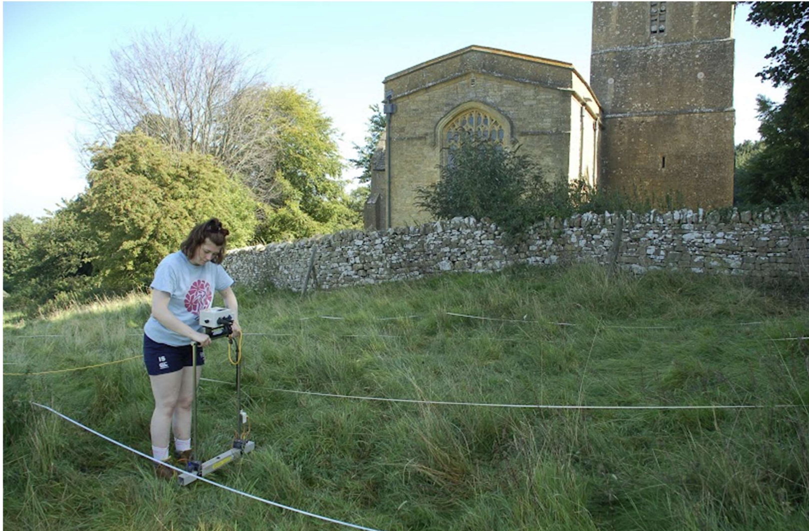
Figure 33: Earth resistance survey being carried out in Area A, immediately west of St Nicholas' churchyard.
